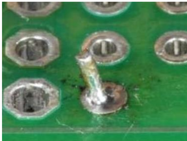
Figure 12: Solder starving. Lack of solder around the area.
