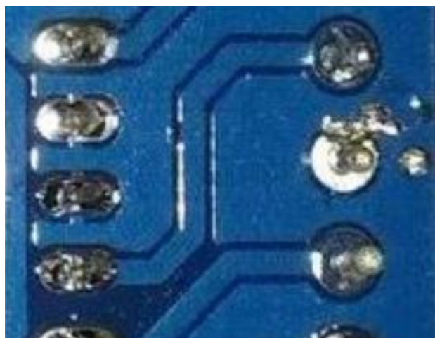
Figure 17: Stray solder pads spatters
