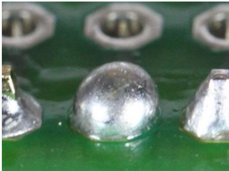
Figure 13: Excess solder and blob formation.
