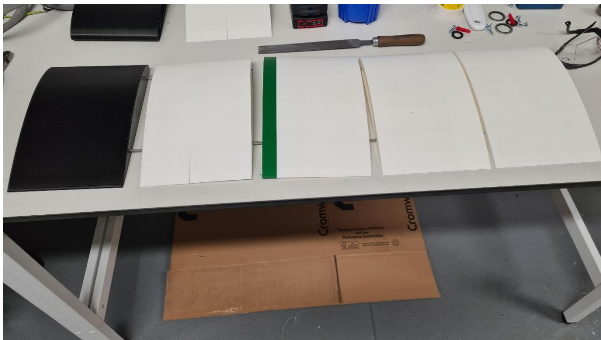
This is to display that the steel rods in between each wing part was inserted and then glued to ensure that it did not break during the experimentation.
